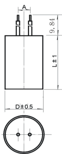
Dry Type Capacitor with Leads
